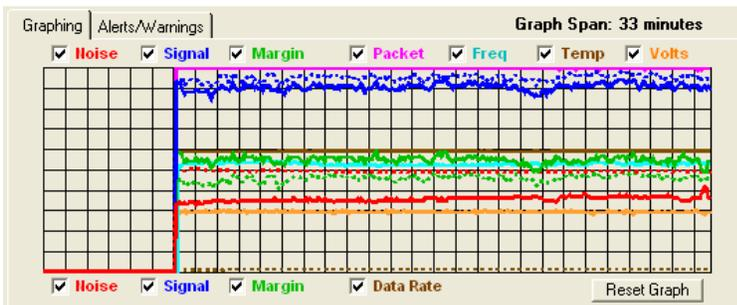
The Noise, Signal and Margin check boxes appear twice. If you select the check boxes above the graph, the system will illustrate the inbound Noise, Signal and/or Margin as a solid line. If you select the check boxes below the graph, the system will display the outbound Noise, Signal and/or Margin as a dashed line.
