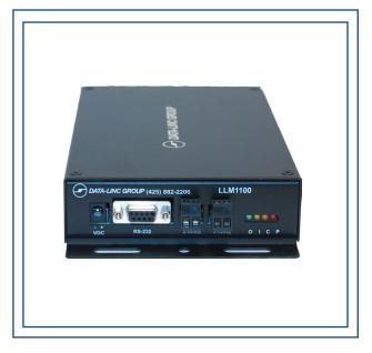
Data-Linc Group's LLM1100 is a Bell 202 (CCITT V.23 optional) 1200 baud modem. It can be easily configured for simplex (bit mode), half-duplex and full-duplex operation. The LLM1100 is designed to be used on private, leased nonswitched telephone lines or any dedicated two-conductor wire (twisted or untwisted, shielded or unshielded).
