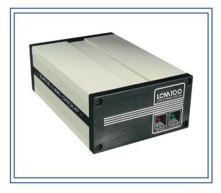
The LCM100 Line Carrier Modem sends and receives digital data over power lines in a facility. It permits full-duplex asynchronous data transmission over 120 VAC (higher voltage options available) power lines at data rates up to 9600 baud. The LCM eliminates costly dedicated cable installations for significant savings. The LCM100 utilizes high frequency FSK for exceptional immunity to inductively coupled industrial electromagnetic interference, resulting in high data reliability.
