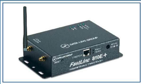
The *FastLinc*™ Family of high speed Industrial Ethernet Wireless Modems provide secure wireless communications using 2.4 GHz direct sequence technology available in stand-alone Ethernet (FLC810E+ and FLC820G) and PCMCIA card (FLC800C+) models as well as the 900 MHz OFDM Ethernet FLC910E modem. With an output power much higher than commercial 802.11b products, the FLC810E+ provides longer outdoor range and broader indoor coverage.
