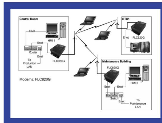
Diagram 4 An equipment arrangement for a multi-drop high speed wireless system which includes laptop computer wireless integration utilizing.
