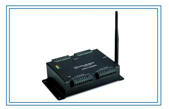
The Data-Linc Group DD1000 and DDAA1000 wireless multiplexers offer applications the ability to transmit 4-20 mA and or discrete signals without the cost or inconvenience of adding wires or additional devices
