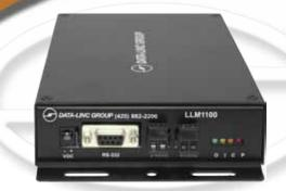
Data-Linc Group's LLM1100 is a Bell 202 (CCITT V.23 optional) 1200 baud modem. It can be easily configured for simplex (bit mode), half-duplex and full-duplex operation. The LLM1100 is designed to be used on private, leased non-switched telephone lines or any dedicated two-conductor wire (twisted or untwisted, shielded or unshielded).
